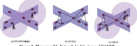
Figure 1: Three possible Network Architectures of VANETs.
